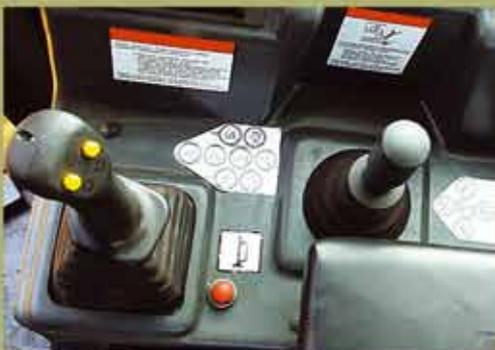
Various blade control levers are used for distinct work equipment specifications (tilt only, tilt/pitch or 6-way blade). Pilot operated hydraulic controls are offered as standard. The right hand ergonomical lever controls raise and lower of the ripper.
