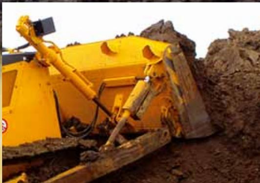
Semi-U blades of 5.7 cu.m (7.45 cu.yd) for STD & LT track frame and 5.95 cu.m (7.8 cu.yd) for WT version, combine penetration ability of straight blade with increased capacity provided by short wings. The blades equipped with tilt, may be additionally offered with tilt/pitch option.
