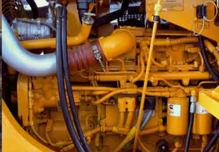
Cummins QSC8.3 engine meets U.S. EPA Tier 3 and EU Stage IIIA emissions standards. The QSC advanced electronics provide enhanced engine performance with higher torque and better throttle response at every rpm. With its ideal combination of electronic controls and durable block design, this engine is ready to meet even toughest machine work conditions. Long maintenance intervals, better cold starting and quieter operation provide improved operator comfort.
