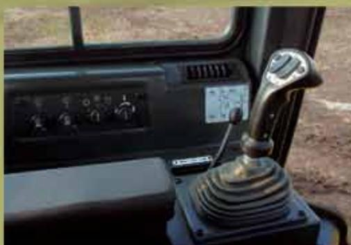
The left hand joystick controls transmission and steering drive for up and down shifting, steering Hi/Lo selection and LH/RH gradual turn. Preset travel speed selection and auto – downshift provide comfortable operation and high productivity without manual downshifting.
