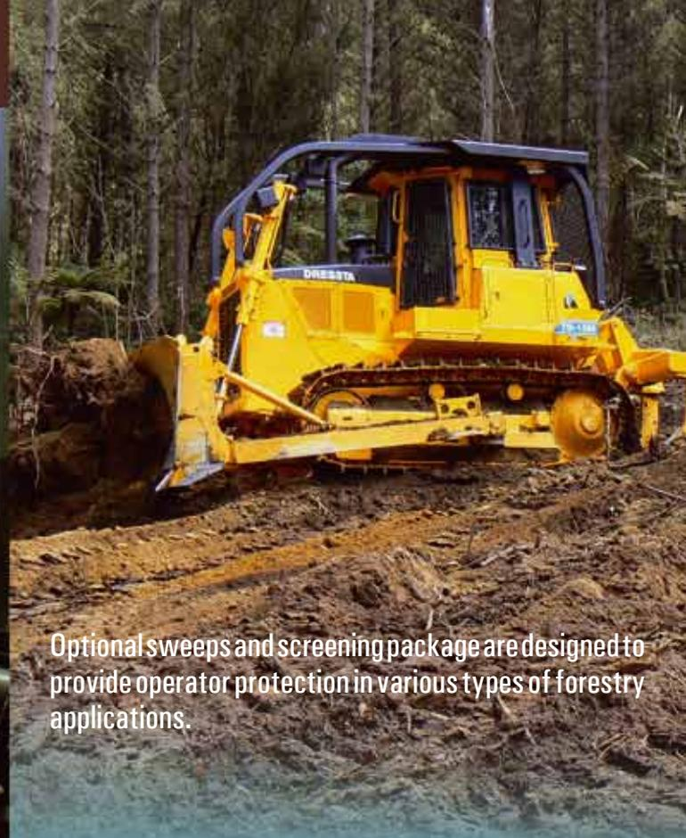
Optional sweeps and screening package are designed to provide operator protection in various types of forestry applications.
