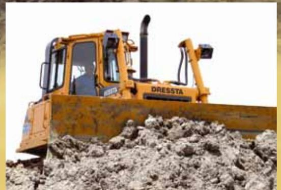
Angle blade of 3.8 cu.m (5 cu.yd) used with STD & LT track frame, is ideal for side-casting, backfilling, cutting ditches or setting a final grade by reducing amount of maneuvering required to do these jobs. 2-cylinder blade tilt is offered as standard.
