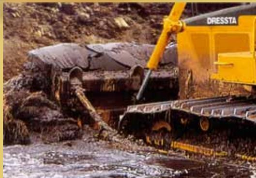
Straight blade of 3.6 cu.m (4.7 cu.yd) used with 2.16 m (85 in) gauge and 940 mm (37 in) track shoes (LGP) is designed for soft, swampy areas. This blade is equipped with hydraulic tilt cylinder to perform efficiently landscaping operations.
