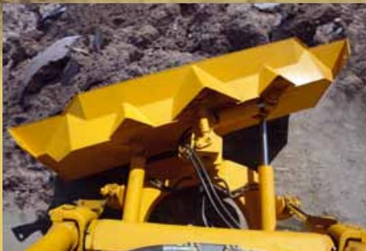
6-way hydraulic angle blades of 3.8 cu.m (5 cu.yd) used with wide track (WT) and 4.0 cu.m (5.2 cu.yd) used with low ground pressure track (LGP) are applicable for versatile operations such as finish grading, spreading material and light land clearing.
